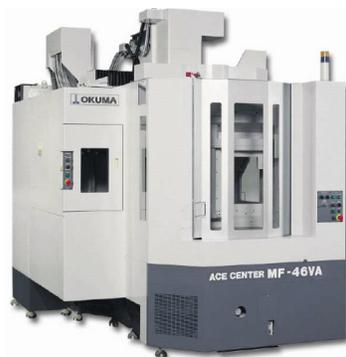
[Photo] An example of one of the Okuma machining centers used to drill holes and deburr them using the OrbiTool.
