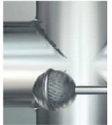
One aspect that must be monitored particularly carefully in this process is drill wear. If the drill is pushed too far in its tool life, the size of the attached swarf and the pushed burr that is generated when the drill breaks through into the central bore become too large for the OrbiTool to remove within the time restraints governing the whole process.
