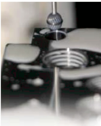
After the work is completed: at Festo, Orbitool deburrer gently chamfers the edges on the bore hole interface.
