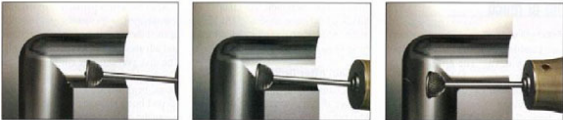
An in-line tool allows drilled cross-holes to be deburred without moving parts to another area of the shop.
