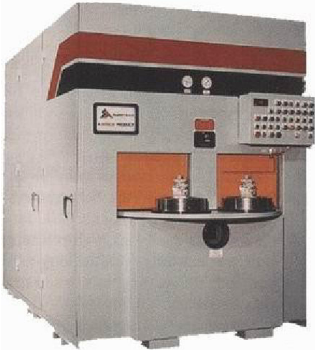
A machine for deburring via the thermal energy method vaporizes burrs with a short burst of intense heat.
